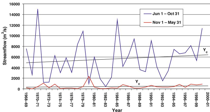
**Fig. 4.4** Trend of monsoon and non-monsoon discharge of the lower Damodar River below the Durgapur Barrage (Data source: Appendix B)
