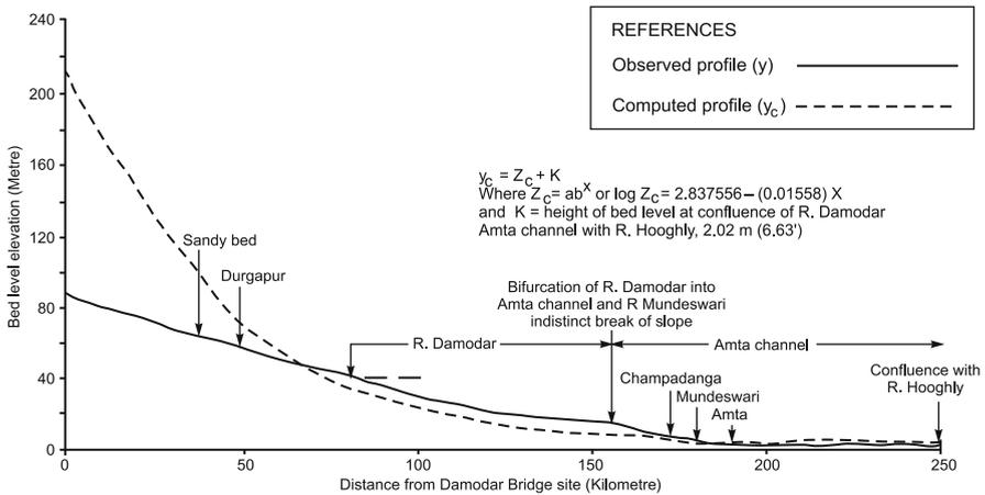
Fig. 4.17 The long profile of the Damodar river (Source: P.K. Sen)
