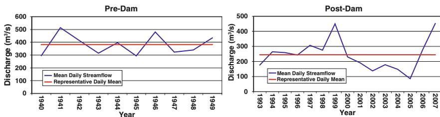
**Fig. 4.1** Characteristics of daily discharge and representative daily average discharge of the lower Damodar River at Rhondia in pre-dam (1940–1949) and post-dam (1993–2007) periods
