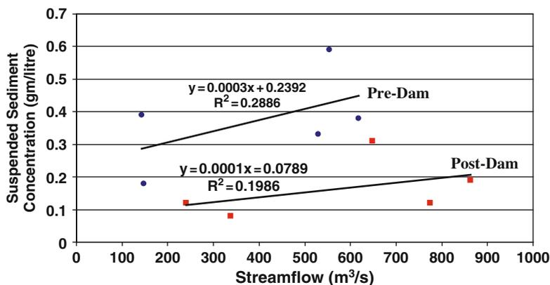
**Fig. 4.14** Linear regression of average monsoon discharge and suspended sediment concentration at Damodar bridge site on the Damodar River in pre-dam and post-dam periods. Data source: Hydraulic Data Division, DVC Maithon
