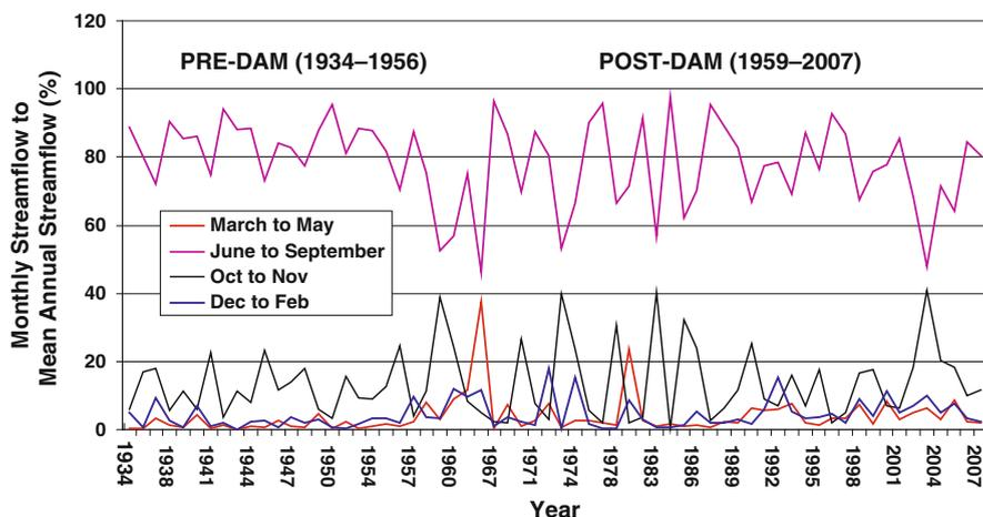
**Fig. 4.3** Discharge characteristics of the lower Damodar River at Rhondia in pre-dam (1934–1956) and post-dam (1959–2007) periods (percentage of streamflow with respect to mean annual total streamflow). Data source: Appendix C
