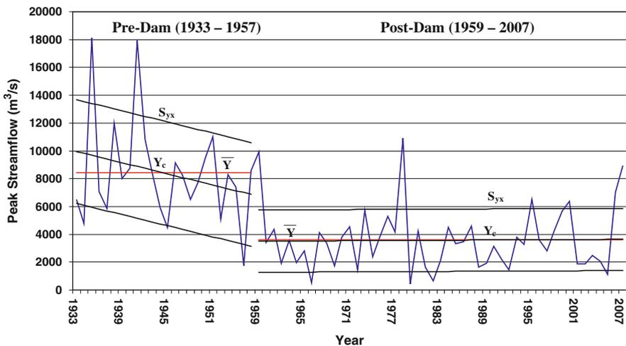
Fig. 4.7 Trend of peak flow of the lower Damodar River in pre-dam and post-dam periods
