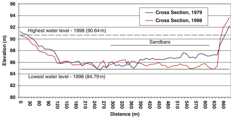
**Fig. 4.15** Cross sections of the Damodar River at 36 m downstream from Damodar bridge site (surveyed on 5-9-79 & 4-23-98). Data Source: Hydraulic Data Division, DVC Maithon
