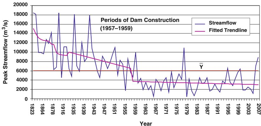
Fig. 4.6 Peak streamflow characteristics of the lower Damodar River at Raniganj (data shown before 1933) and at Rhondia (data shown from 1933 to 2007). Data Source: Refer to Appendix F
